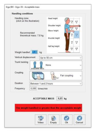
Figure 6. Ergo+50 - Calculation of the acceptable mass
